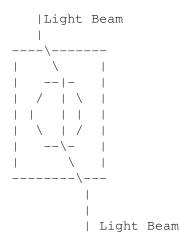
In the above, we have the box and sphere. The lights comes in from the back (it doesn't matter which directio), refracts at the air/glass interface, and travels in the box. Then refracts at the glass/air interface of the box/sphere. Then again at the air/glass, and finally at the glass/air at the front of the box. It does not matter that this is not "a true solid" as refraction only happen at the interface. Hope all this helps!
